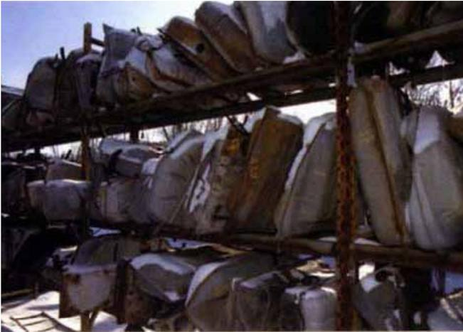
Fuel tanks are dangerous to work on or store; whenever possible replace a tank and never work on a tank if you are not fully qualified to do so.
