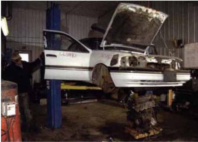
Removing engines exposes you to hazards from gasoline, solvents, other flammables, oils, other lubricants, Freon and sulphuric acid as well as improper use of tools and awkward positioning.
