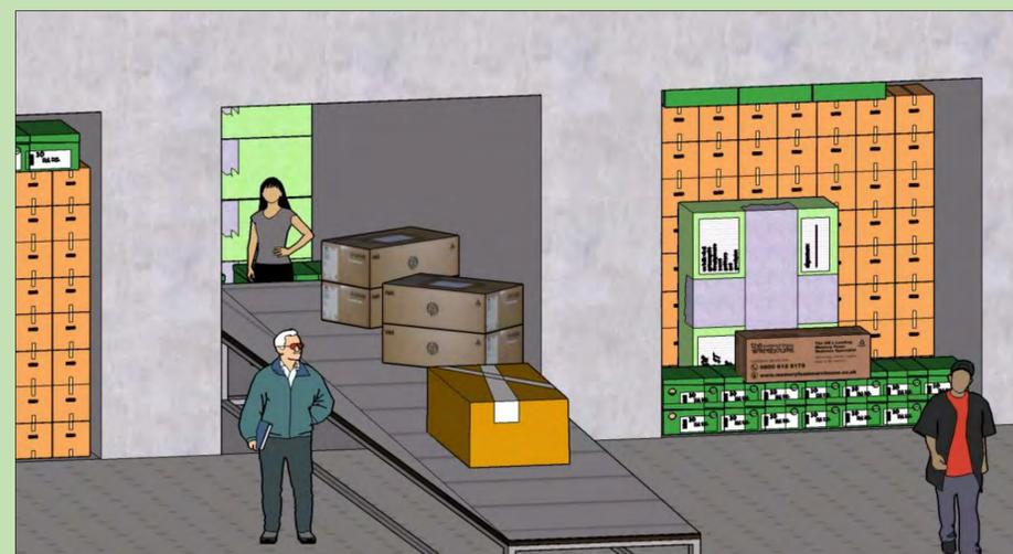
Figure 7. The system that is currently in place. Off-loaders are required to enter the trailers to manually remove the packages. This increases the risk of the development of musculoskeletal disorders from poor ergonomic design. The risk is also increased by the various other environmental hazards that are present in the trailer.
