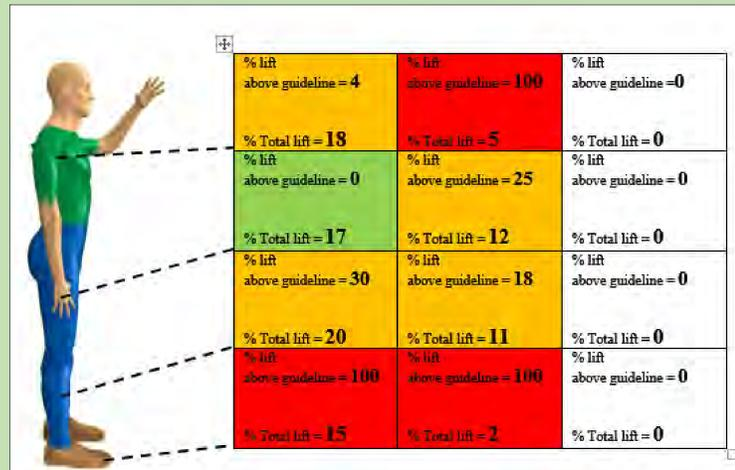
Figure 3. ACGIH Threshold Limit Values (TLVs) for each lifting zone and the average percentage of lifts in each zone.
