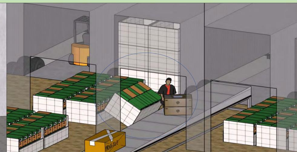
Figure 8. The new proposed design is a semi-automated system that reduces human engagement with the use of loading bins and forklifts to load the trailers. Workers no longer need to enter the trailer to off-load the packages.
