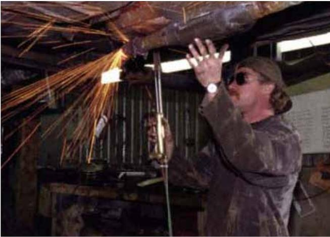
When removing parts with an oxyacetylene torch you are at risk from welding fumes, flames, and compressed gases, as well as from sharp edges in the parts and from having to work in an awkward position.
