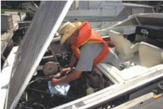
When changing oil in a boat, beware of hot oil, slips and falls due to spills, MSDs, and possibly serious crushing injuries if the boat falls from a hoist or blocks.
